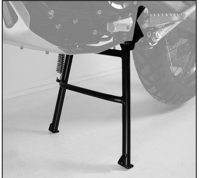
**Please check now the function of your centre stand and control all assembled screw connections for tightness! Use the side stand as a help to get the motorcycle onto the centre stand.**
