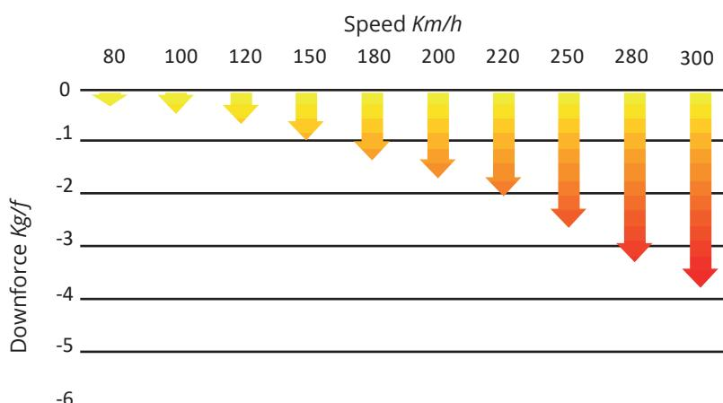
The Downforce that the spoilers generates raises potentially as the speed increases, at 200 km/h we get 1,6 Kg/f.
