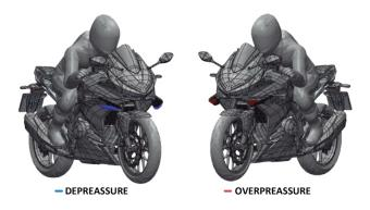
Due to its angles and frontal surface, it creates an overpressure on the top of the spoiler. The turbulance create below, generates a difference of pressure between the upper and lower part of the spoiler. Which ultimately generates the aerodynamic downforce.
